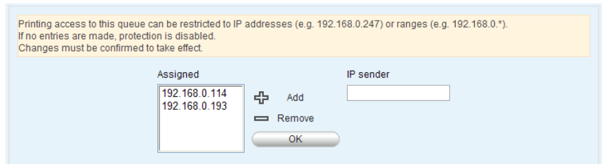
Fig. 15: ISD Control Center - Queue Access Control
