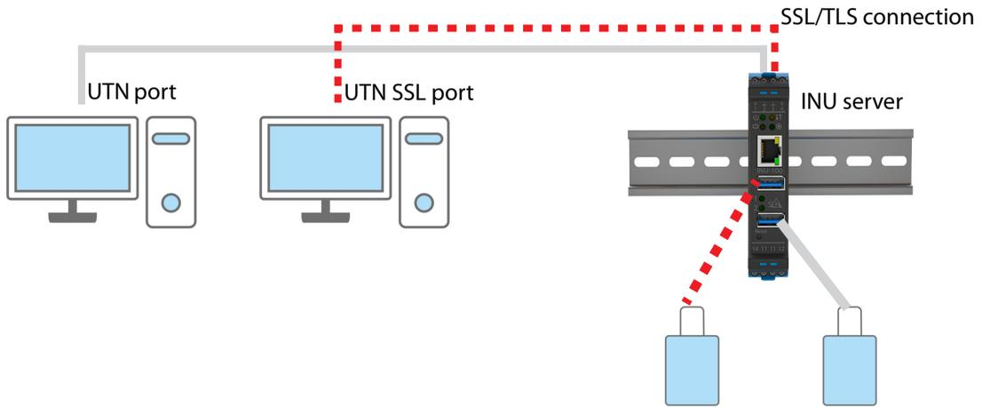
Figure 7: INU Server – SSL/TLS connection in the network
