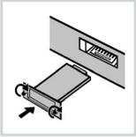
3. Slide the PS107 into the Type B interface.
